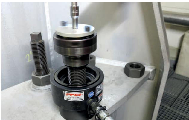
The flexible change bushing gets run down onto the BTC body.
